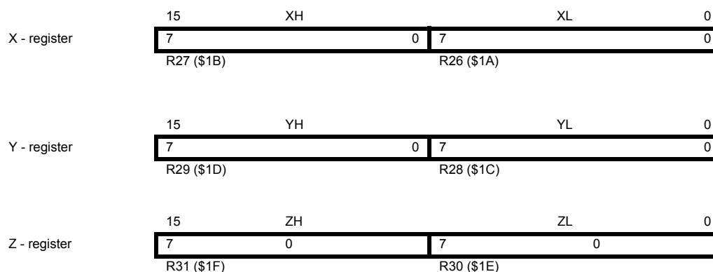
Figure 7-3. The X-, Y-, and Z-registers
