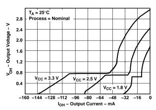
Figure 1. Output Voltage vs Output Current
