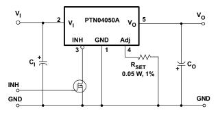
Figure 17. Inhibit Circuit
