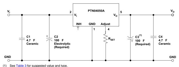
Figure 19. Adding High-Frequency Bypass Capacitors to the Input and Output
