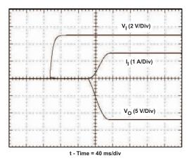
Figure 16. Power-Up Waveforms
