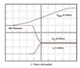
Figure 18. Inhibit Waveform
