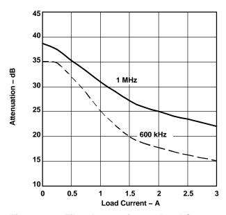
Figure 21.  $\pi$ -Filter Attenuation vs. Load Current
