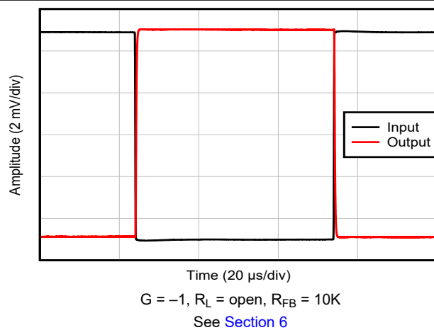
Figure 5-27. Small-Signal Step Response, G = -1
