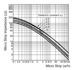
For example, when creating 50-Ω lines using a glass epoxy base with a thickness of 1.6 mm, the above graph will yield a w/h ratio of 1.7 for a dielectric constant of 4.8. Since the base thickness is 1.6 mm, the width will be  $h \times 1.7 \approx 2.7$  mm.
