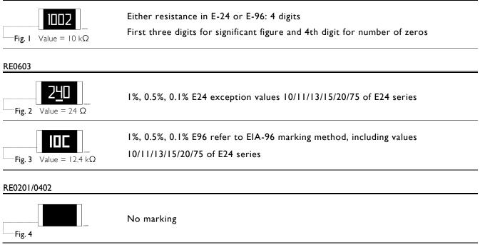
For further marking information, please see special data sheet "Chip resistors marking".
