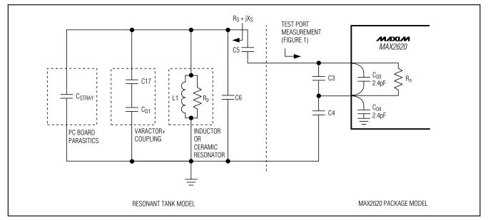
Figure 5. Electrical Model of MAX2620 Circuit
