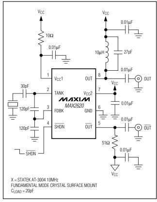
Figure 4. 10MHz Crystal Oscillator
