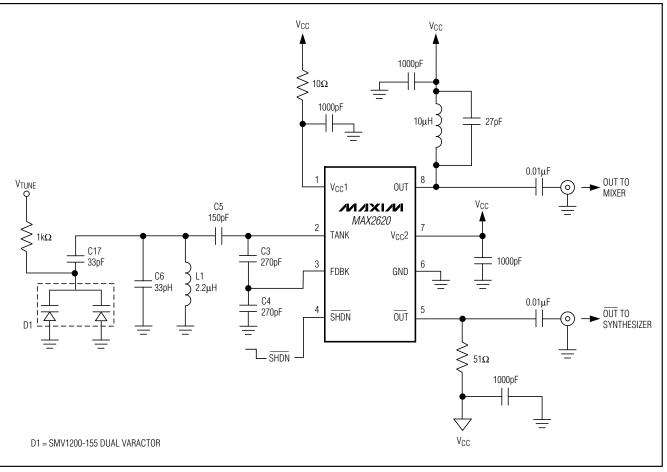
Figure 3. 10MHz VCO LC Resonator
