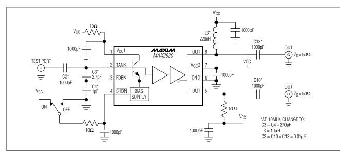
Figure 1. 900MHz Test Circuit
