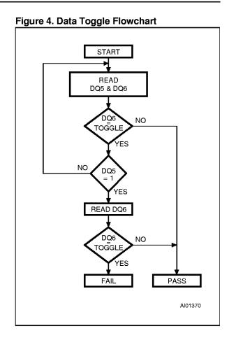
gram, Block Erase or Chip Erase operation fails to write the correct data to the memory. If the Error Bit is set a Read/Reset command must be issued before other commands are issued. The Error bit is output on DQ5 when the Status Register is read.
