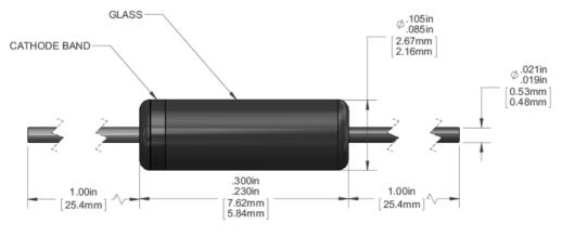
Lead Material: copper clad steel
