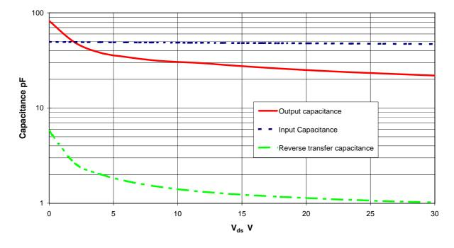
Figure 5 – Typical CV Characteristics.
