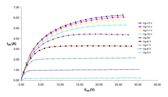
Figure 4 – Typical IV Characteristics.
