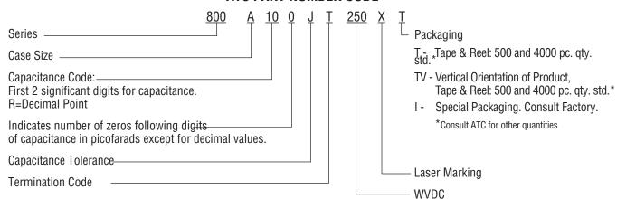
The above part number refers to a 800 A Series (case size A) 10 pF capacitor, J tolerance (±5%), 150 WVDC, with T termination (Tin Plated over Nickel Barrier, RoHS Compliant), laser marking and tape and reel packaging.
